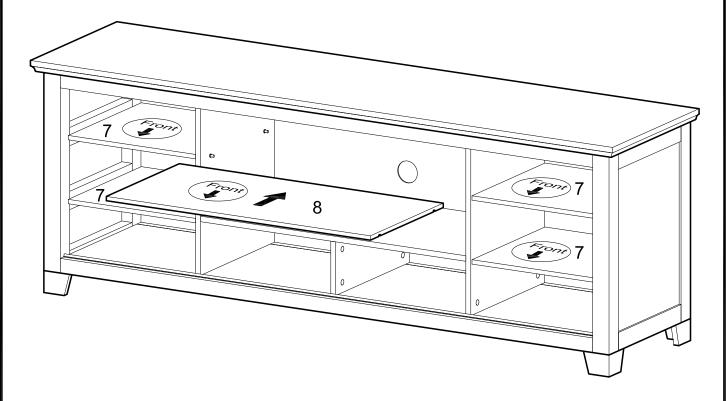
Carefully place shelves (7,8) into the console. Note the direction of the shelves as shown in the diagram. Shelves will rest on the shelf support pins.
